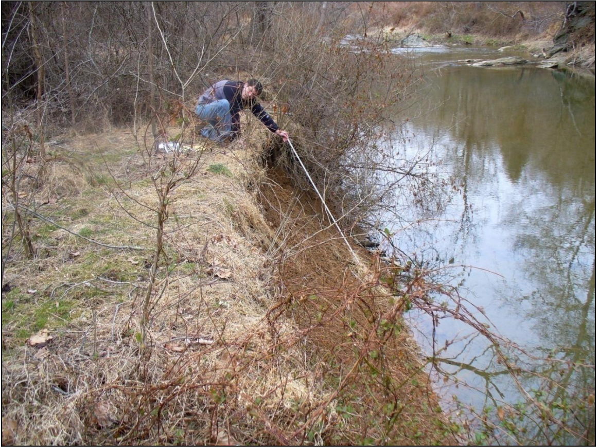
Figure 4: An actively eroding stream bank directly upstream from a breached mill dam on Gunpowder Falls.
