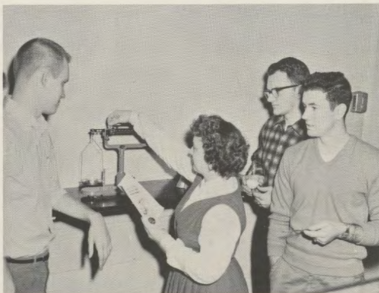
Miss Janice Griewahn demonstrates the use of a Specific Gravity Balance to Ronald Windle, Roger Steele, and Ronald Broadwater in General Chemistry.
