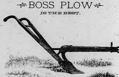
1st. It has curved iron standard with flanges to hold the beam, and a simple deear end of beam to make plow run deep or shallow. 2d. It can be made to go in the ground in any weather and get double wear out of a point.
