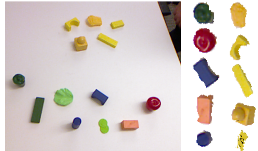
Fig. 4: An example of an RGB-D object identification scene. Columns on the right show examples of segmented objects. The far right column shows objects identified by the sentence “These are various types of yellow colored objects”; the center column shows non-selected objects. The correct associated RCL interpretation is \lambda.x(\text{obj-color } x, \text{color-yellow}) .
