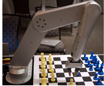
Fig. 1: The mid-cost Gambit manipulator arm was designed for small-scale tabletop manipulation tasks. Here, it plays chess against a human opponent.
