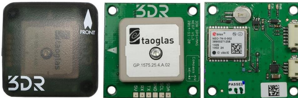
FIGURE 3.6 EXTERNAL, INTERNAL TOP AND BOTTOM VIEWS OF UBLOCK GPS MODULE [14]
