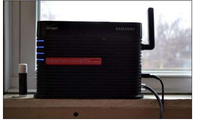
Femtocells are devices same as modems. It could be connected to service provider's network through broadband or DSL cable. Standard edition handles up to 8 mobile devices. There are no worries of interference, building obstacles faced in general scenario, low power, handover problems.
