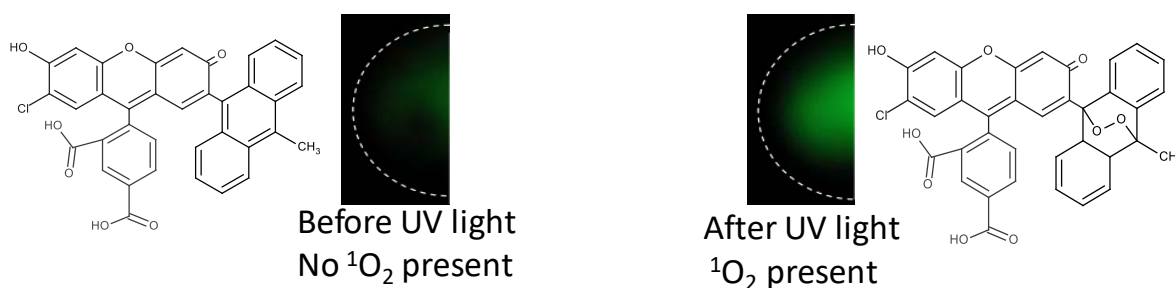
Figure 1.10 (A) Singlet oxygen sensor green (SG) reagent before UV light exposure and no ^1\text{O}_2 present. (B) SG after UV light exposure and ^1\text{O}_2 present. Adapted from 59.
