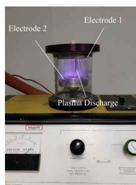
Figure 1: Technics Hummer II sputtering chamber triggering a DC cold plasma discharge at 30mA that ionizes the Titan-simulated N_2 - CH_4 (90%-10%) gas mixture to produce tholins after several days.
