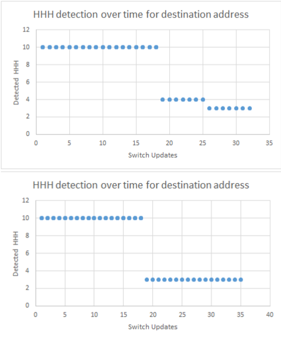
FIG. 5.1. The results from the targeted heavy flow traffic simulation on both SDN configurations. The upper graph represents raw traffic statistics analyzed by the HHH algorithm, while the lower figure represents analysis done by flow
