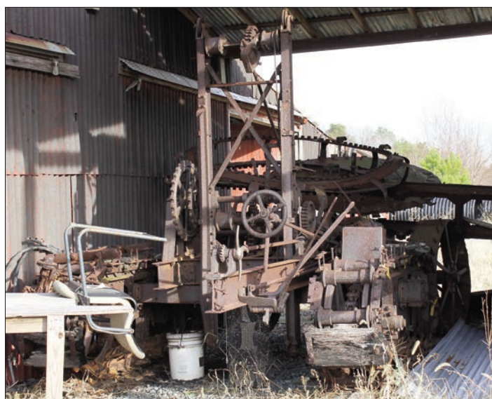
Trenching machine that was used on the Gibbs’ marsh to cut trenches to place boards upright in the ground to “corral” the muskrats. This machine is now at the Blackwater Refuge. Courtesy of Tom Bradshaw.
