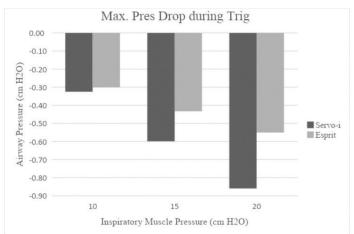
**Figure 3.** Mean Maximum Pressure Drop during Triggering. This figure displays the inspiratory muscle workload required to trigger ventilator breath delivery. The Maquet Servo-i measures were more negative, demonstrating increased workload for patients.
