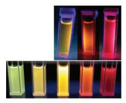
Figure 3: CuInS<sub>2</sub> quantum dots in our lab (top) against CuInS<sub>2</sub> quantum dots claimed from research by Chen et al. (bottom) (2013) shown glowing under ultraviolet light.
