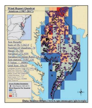
Figure 3 gives a visual description of the wind report quadrat analysis. Each confirmed report is shown in the location it occurred. Quadrat analysis resulted in a VMR = 16.262 (p < 0.00001) indicating statistically significant clustering of wind reports. The superimposed quadrats were color-coded based on the number of reports, which revealed that the vast majority of the reports occurred north of the Delaware state-line.
