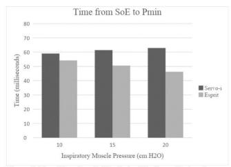
**Figure 2.** Mean Time from SoE to Pmin. This figure displays the average time from the start of an inspiratory effort to the lowest airway pressure required to trigger ventilator breath delivery. The Respironics Esprit mechanical ventilator outperforms the Maquet Servo-i under each measure of inspiratory muscle pressure, suggesting that it is superior in spontaneous breath detection.
