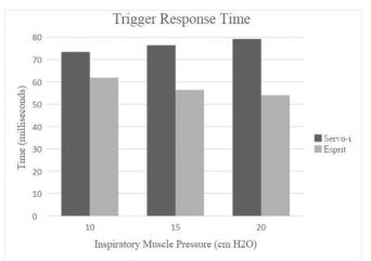
**Figure 1.** Mean Trigger Response Time. This figure displays the average time for the pressure to fall and rise back to baseline during an inspiratory effort. The Esprit TRT is lower in all three measures of inspiratory muscle pressure. This suggests that the Esprit is more capable of detecting effort and applying initial flow over the Servo-i.
