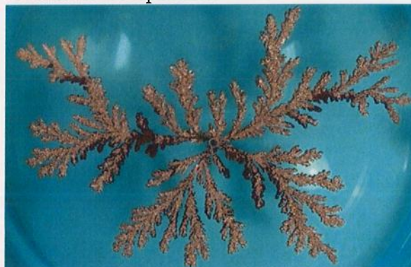
Figure 2: A copper cluster formed by Electrochemical Deposition
