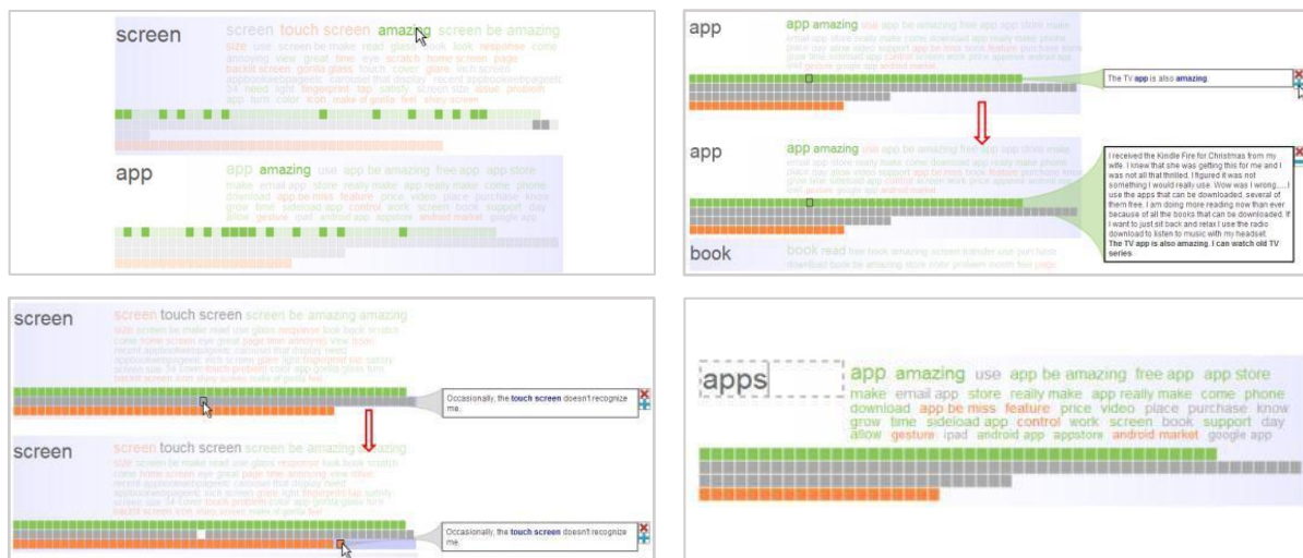
Figure 6. The OpinionBlocks interface. Top Left: Hovering over a keyword reveals which colored comment blocks contain the selected phrase. Top Right: Clicking on a block reveals a snippet of text and selecting the plus icon reveals the entire comment. Bottom Left: Comments can be dragged into other colored rows to change their sentiment rating. Bottom Right: Titles of categories can be changed by clicking them to edit (Hu, et al., 2013).
