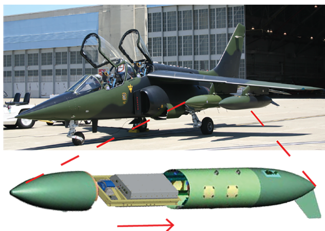
Figure 10. The COFFEE instrument, installed in its AJAX pod rack, is mounted into the mid-body of the inboard left pod.
