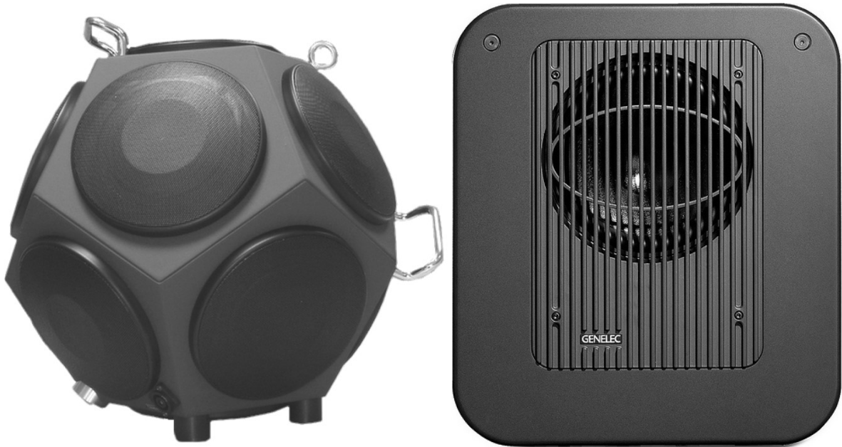
Figure 4: An image of the audio equipment used to generate the steady-state noise stimuli. The dodecahedron loudspeaker system is on the left and the subwoofer is on the right.
