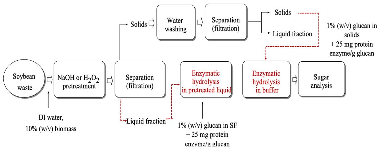
Figure 4. The schematic diagram for the enzymatic hydrolysis of hydrothermally pretreated soybean wastes.
