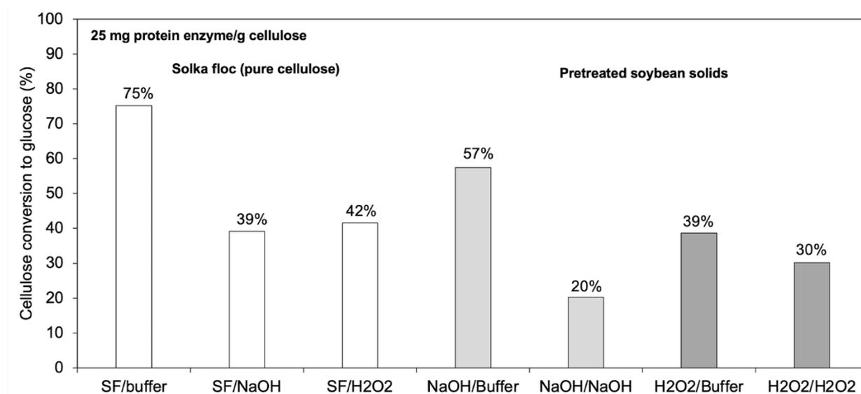
Figure 5. The cellulose conversion to glucose after the enzymatic hydrolysis of H<sub>2</sub>O<sub>2</sub> and NaOH pretreated soybean solids and Solka Floc samples with 25 mg protein enzyme/g cellulose in 10 mL of 50 mM citrate buffer (pH 4.8) or pretreated H<sub>2</sub>O<sub>2</sub> and NaOH liquid. After the enzymatic hydrolysis, the remaining endo-glucanase and  $\beta$ -glucosidase enzyme activity of the Solka Floc and H<sub>2</sub>O<sub>2</sub> or NaOH pretreated samples was measured.
