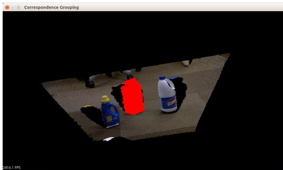
Figure 12: ORC system performing object recognition in scene data
