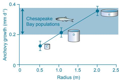
**Figure 61:** Variations in growth rate (mean  $\pm$  SE) of bay anchovy (*Anchoa mitchilli*) with increasing radius of experimental containers. Growth rates were measured as an increase in standard length of fish during period of captivity in container.<sup>35</sup>
