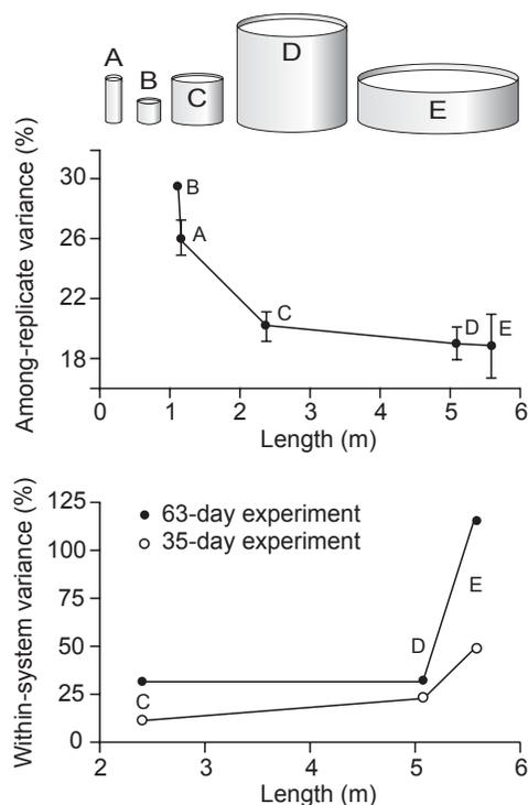
**Figure 63:** Changes in relative variance for measurements of phytoplankton abundance among replicate experimental systems with changes in container size (top panel),<sup>32</sup> and changes in relative variance for zooplankton abundance within experimental systems with changes in container size after 35 and 63 days of experiments (bottom panel).<sup>37,38</sup>
