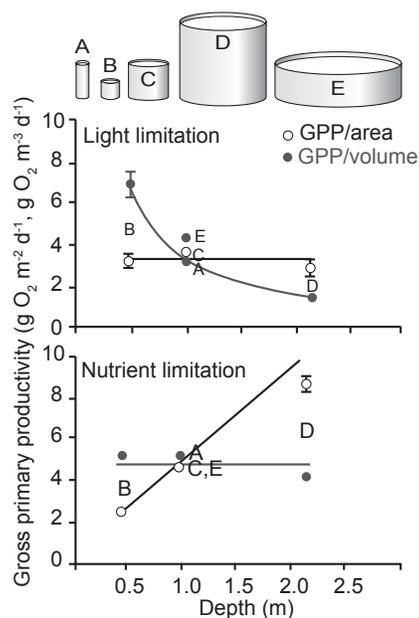
**Figure 53:** Variations in gross primary productivity (GPP) in mesocosms of different depths. Mean GPP values (calculated both per water volume and per water surface area) and water column depth for (top panel) spring experiments under light-limited algal growth conditions and (bottom panel) summer experiments under nutrient-limited growth conditions.
