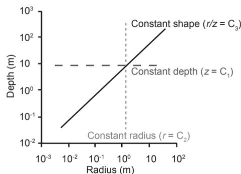
**Figure 51:** Alternative simple relationships by which depth and radius of mesocosms might tend to be related. Constant radius: depth is varied but width (radius) is held constant. Constant depth: radius is varied but depth is held constant. Constant shape: depth and radius are varied in constant proportion to one another. Researchers tend to use containers with relatively constant shape.<sup>20</sup>
