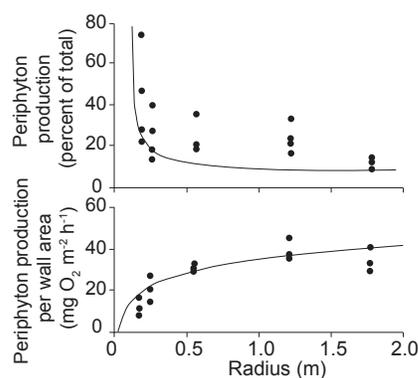
**Figure 60:** Changes in relative contribution of wall periphyton to total gross primary productivity (top panel) and in productivity of wall periphyton per unit of wall area (bottom panel) with mesocosm radius. The curved lines through the data are a least-squares fit using the hypothesized inverse relationship between relative productivity and tank radius  $GPP_{wall}/GPP_{total} = C_3/r$  (top panel), and a best-fit line (bottom panel).<sup>31,33</sup>
