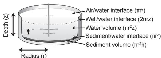
**Figure 50:** Conceptual diagram showing key regions of biogeochemical activity associated with the spatial scales of a pelagic-benthic mesocosm. ( $h$ =sediment depth)
