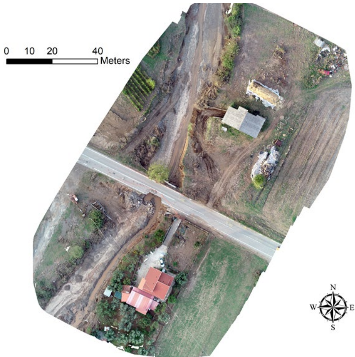
Figure 5.30. UAV-enabled orthophoto of road failure on E.O. Lamia-Karpenisi ( 38.94233611^{\circ}\text{N} , 22.21619722^{\circ}\text{E} )
