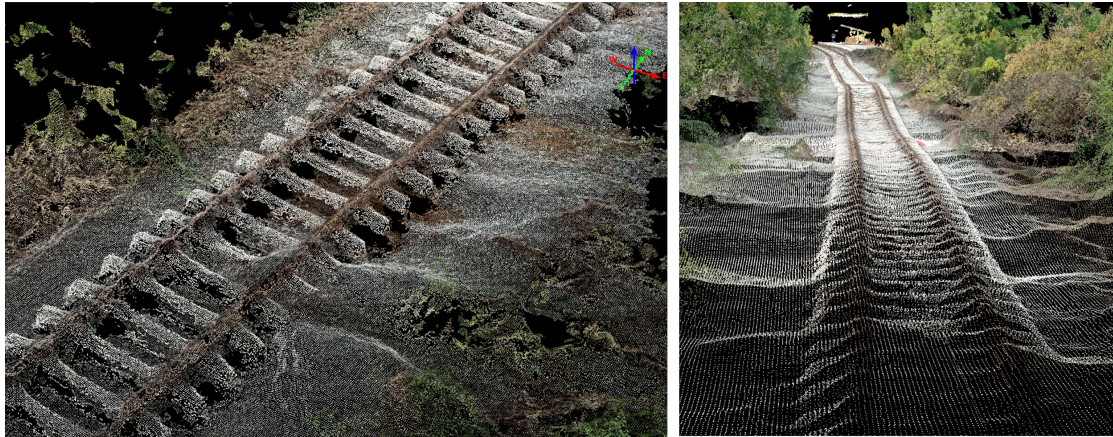
Figure 5.44. 3D Point cloud views of railway ballast breach (left) and rail line deformation (right).
