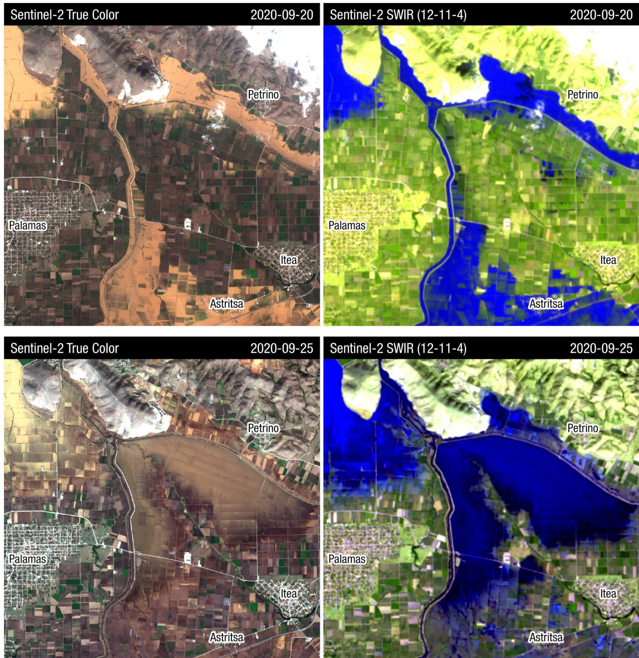
Figure 4.33. Flooded areas from Enipeas and Farsaliotis rivers. Top: Sentinel-2 image (True color and Short-wave infrared composite) on September 20, 2020. Bottom; Sentinel-2 image (True color and Short-wave infrared composite) on September 25, 2020. Accumulation of water east of Palamas occurred in the days following the flood event, as water moved downstream.
