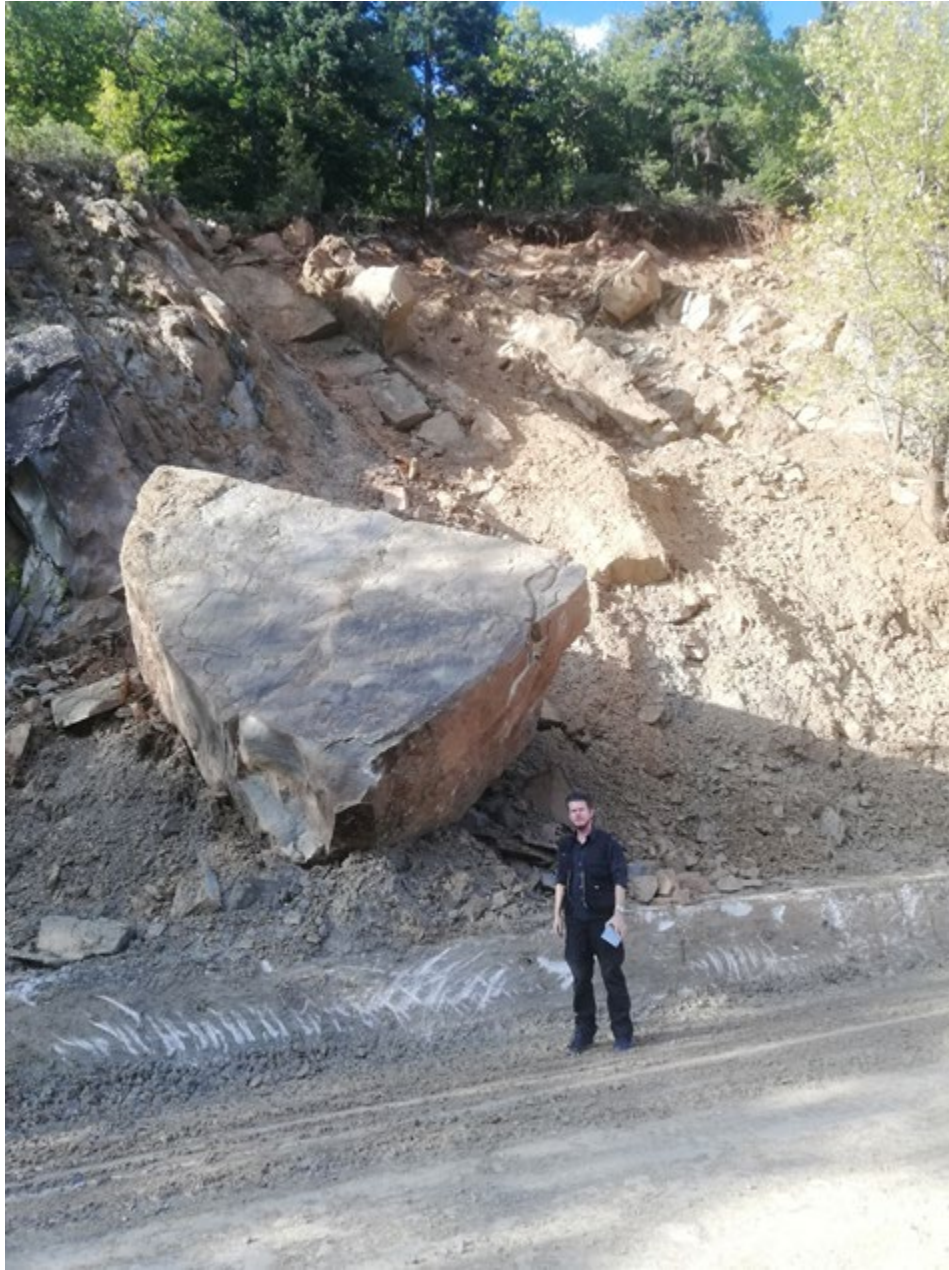
Figure 6.33. Wedge failure mechanism at the area of Belokomiti. (39.25325°N, 21.72192°E)
