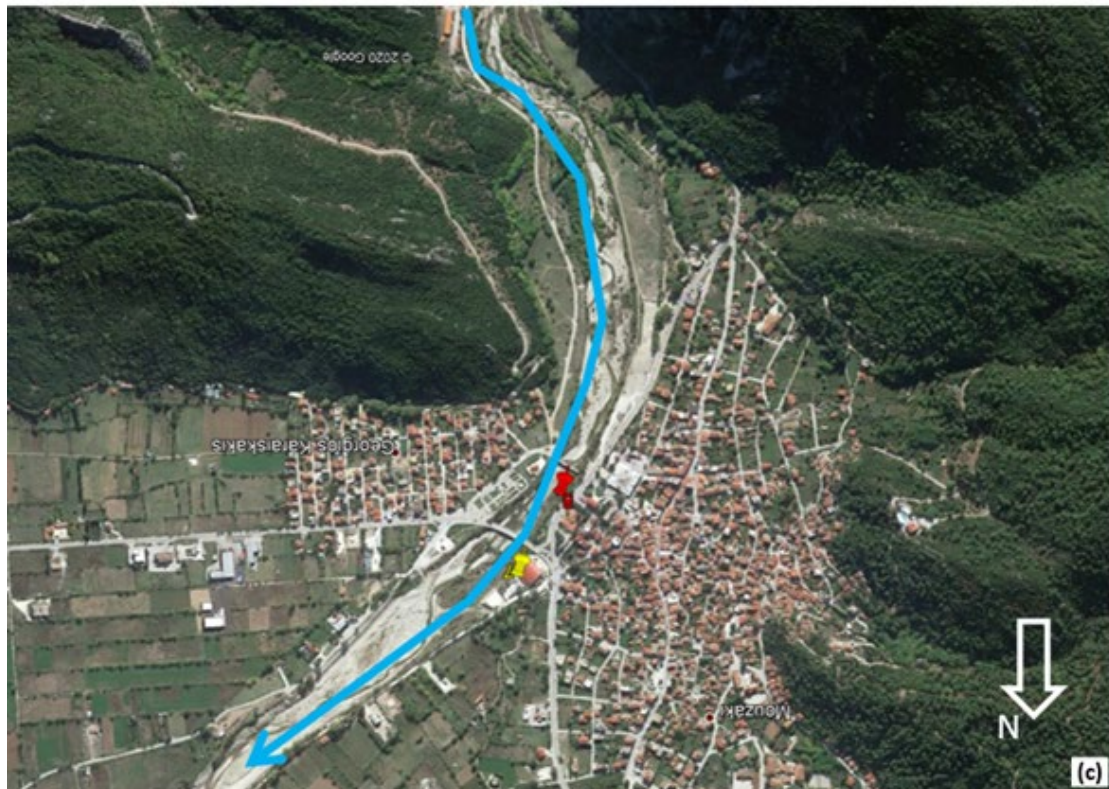
Figure 5.19. (a) Drone footage captured on September 19, 2020 (source: https://www.youtube.com/watch?v=3bqDobqMuC0 ) showing that erosion damage was concentrated on the left (N-W) riverbank while the right (S-E) side remained unaffected; (b) river course geometry that helps explain the scour of the exterior bank of the river..
