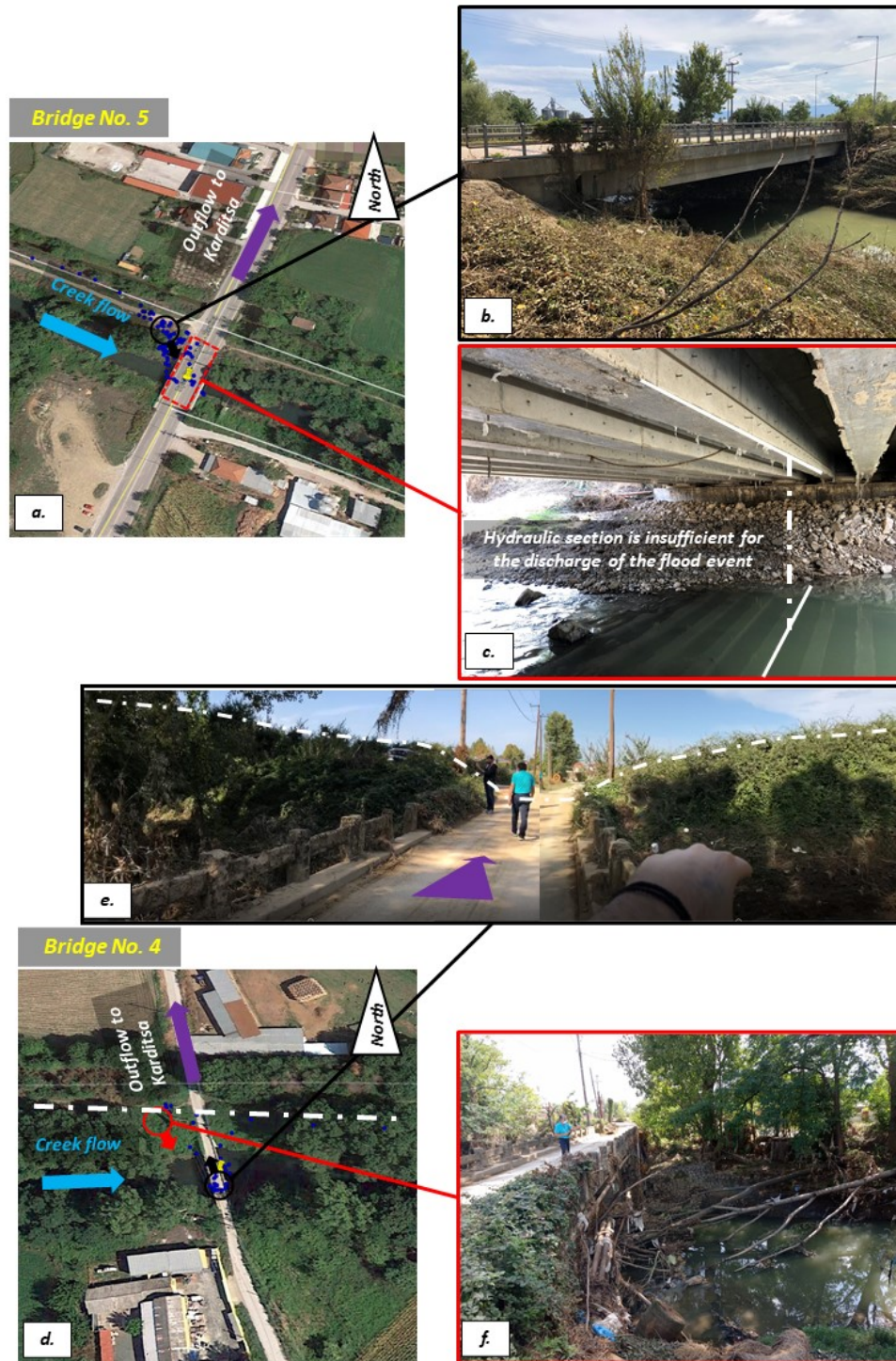
Figure 8.3. (a; b; c) Bridge No. 5 (39.34652222°N; 21.92067222°E): (a) location, (b) section that failed to discharge the flow during the flood event, (c) debris leftovers on the bridge girders (photo taken below the bridge); (d; e; f) Bridge No. 4 (39.348575°N; 21.90459167°E): (d) location, (e) the Flood Protection Levee is lowered at the location of Bridge No. 4, hence leaving a free pass to the flooded water to the north, (f) debris leftovers on the riverbed.
