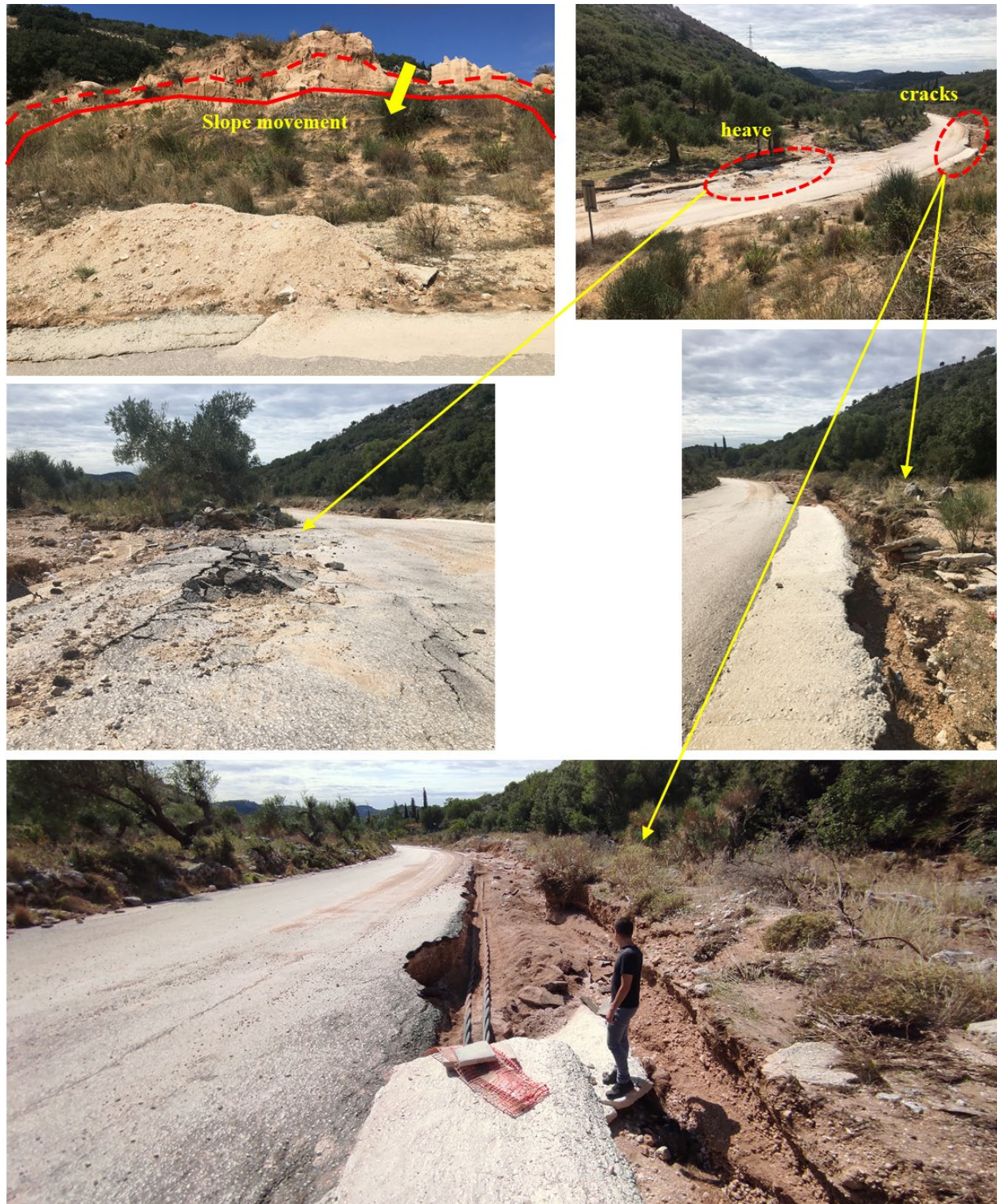
Figure 5.28. Roadside slope failure that led to road heave and cracks along a 150 m stretch (38.201636111°N, 20.502291667°E)
