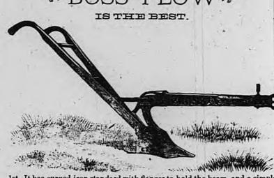
lst. It has curved iron standard with flanges to hold the beam, and a simple de vice under the rear end of beam to make plow run deep or shallow.
