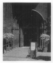
Figure 12. The Smithsonian Institution installed a temporary ramp on its visitor's center to allow adequate time to design an appropriate permanent ramp. Photo: Thomas Jester.
