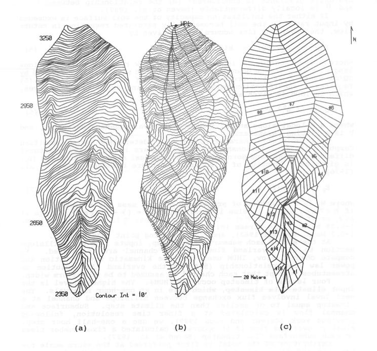
Figure 1. Terrain analysis for WS2 at the Coweeta Hydrologic Laboratory. Shown are: (a) original contour map with stream location and approximate watershed boundaries, (b) "stream tube" delineation using TAPES-C software, (c) resulting hillslope planes fitted (but untransformed) for IHDM4.
