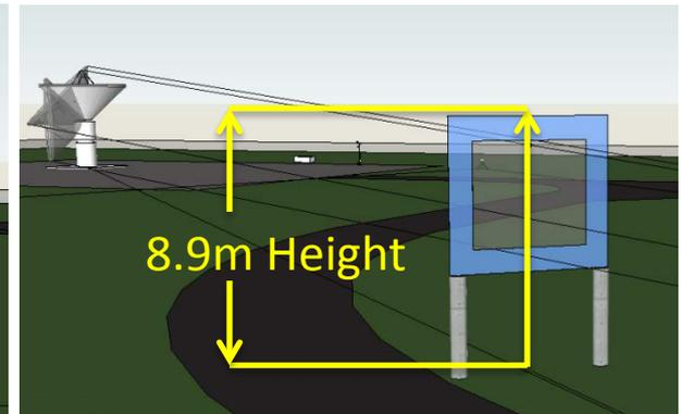
*RFI Blocker size takes into consideration full range of motion of VLBI antenna, and distance to SLR radar. Its centerline is located along the Radar-VLBI baseline.*
