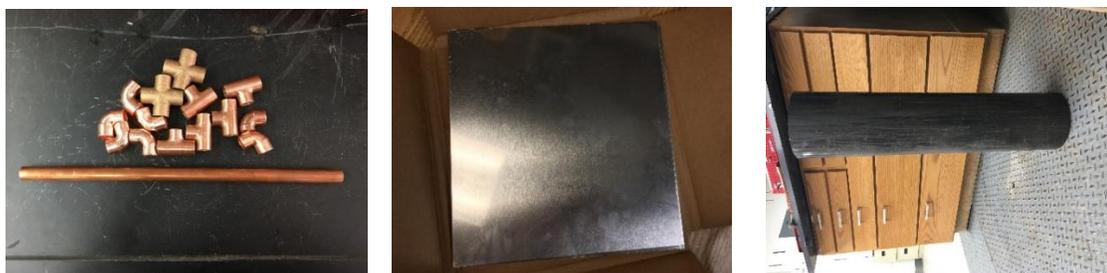
**Figure 5.6: Raw Materials for SHTE Components**
