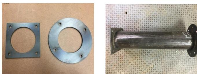
**Figure 5.7: Flanges and Shell of the STHE System**
