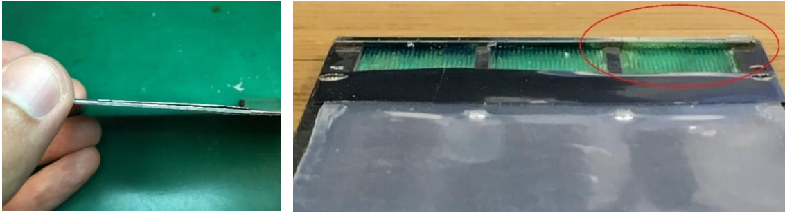
Figure 121: (left) Vikuiti reflector delamination. (right) Missing epoxy is likely the cause for poor polishing and termination.
