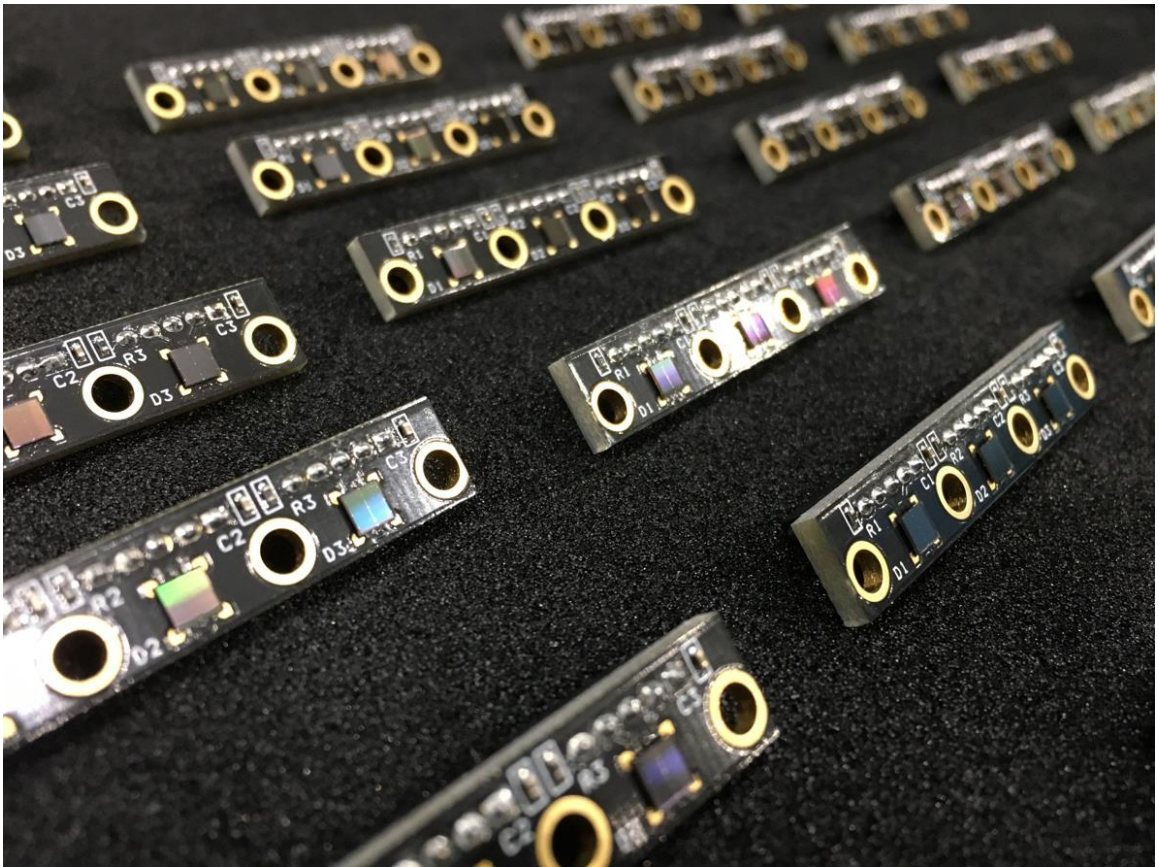
Figure 29: a photograph of SiPMs mounted on PCBs for mounting to face of the WLS fiber block
