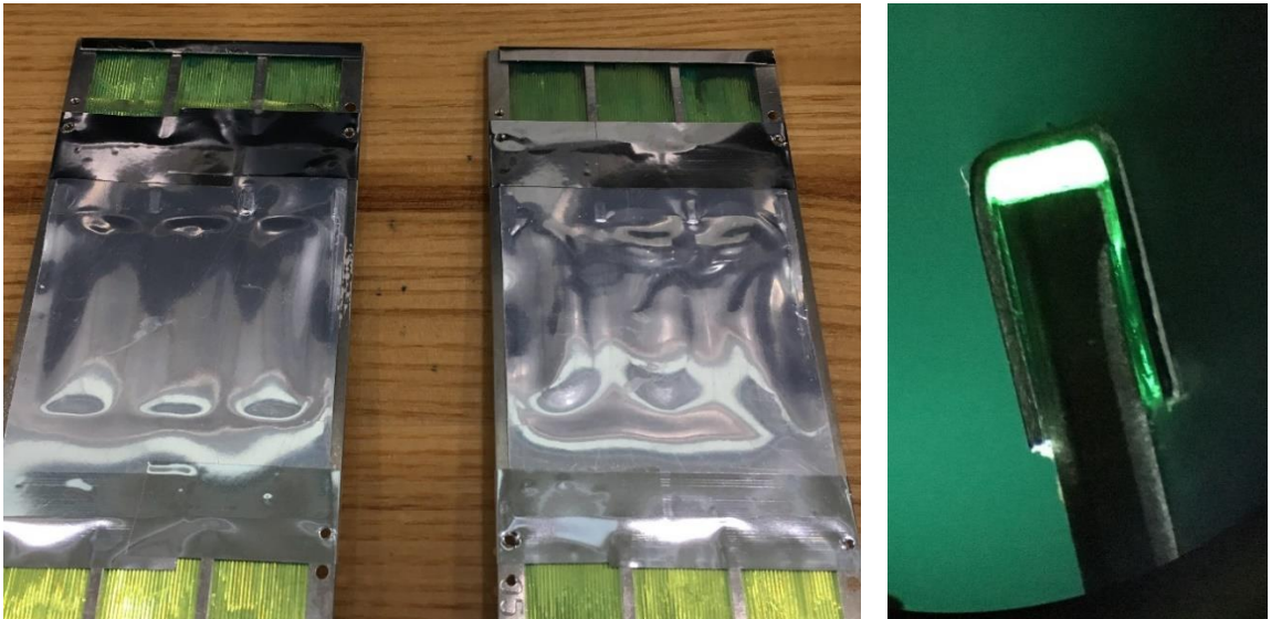
Figure 120: (left) abnormal warping likely caused by scintillator/frame misalignment. (right) gap in end reflector termination.
