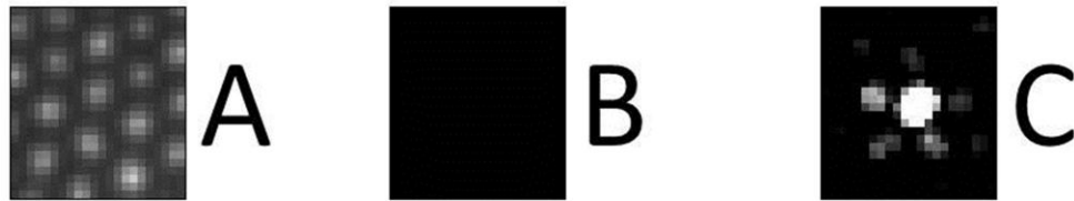
Figure 2.5: White light image of a small area on a fiber bundle (A), fluorescent image of the same bundle that has been dip coated in a quantum dot solution of 6 \times 10^{14} QD/L (B), and a fluorescent image of the same bundle that has been dip-coated in a quantum dot solution of 6 \times 10^{16} QD/ L (C). All images are of the same area and have the same contrast for comparison purposes.
