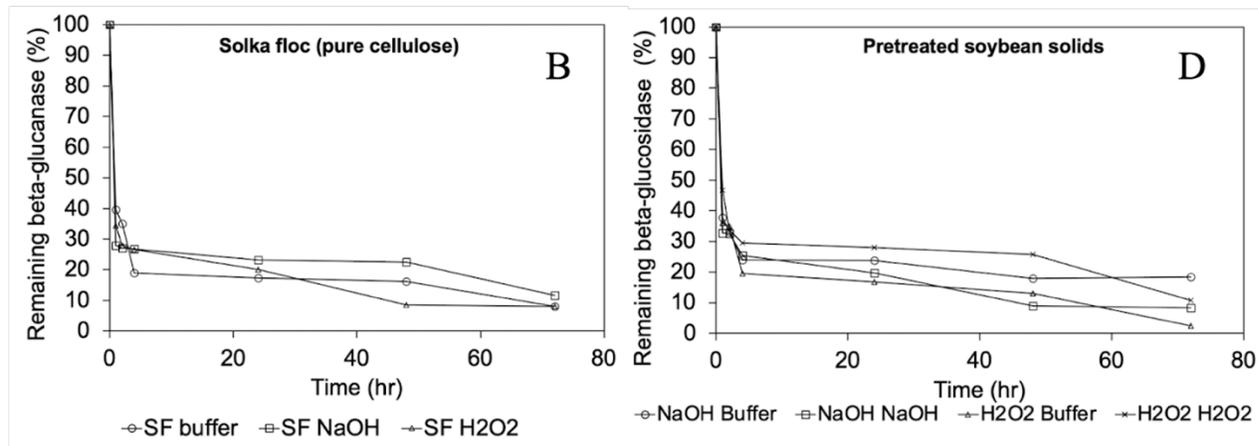
Figure 6. The remaining endo-glucanase and  $\beta$ -glucosidase enzyme activity of the Solka Floc and H<sub>2</sub>O<sub>2</sub> or NaOH pretreated samples was measured using seven sets of the samples in a shaking incubator at 50°C for 72 hrs with Cellic Ctec2 cellulose enzyme. The liquid was extracted from the samples at set intervals, filtered using a syringe, and analyzed with a CellG5 assay reagent kit.
