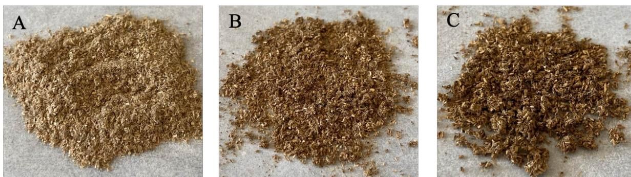
Figure 3. (A) Raw soybean straw, (B)  $H_2O_2$  pretreated, and (C) NaOH pretreated soybean straw solids. Hydrothermal pretreatment decreased the particle size and the chemical composition of raw material.
