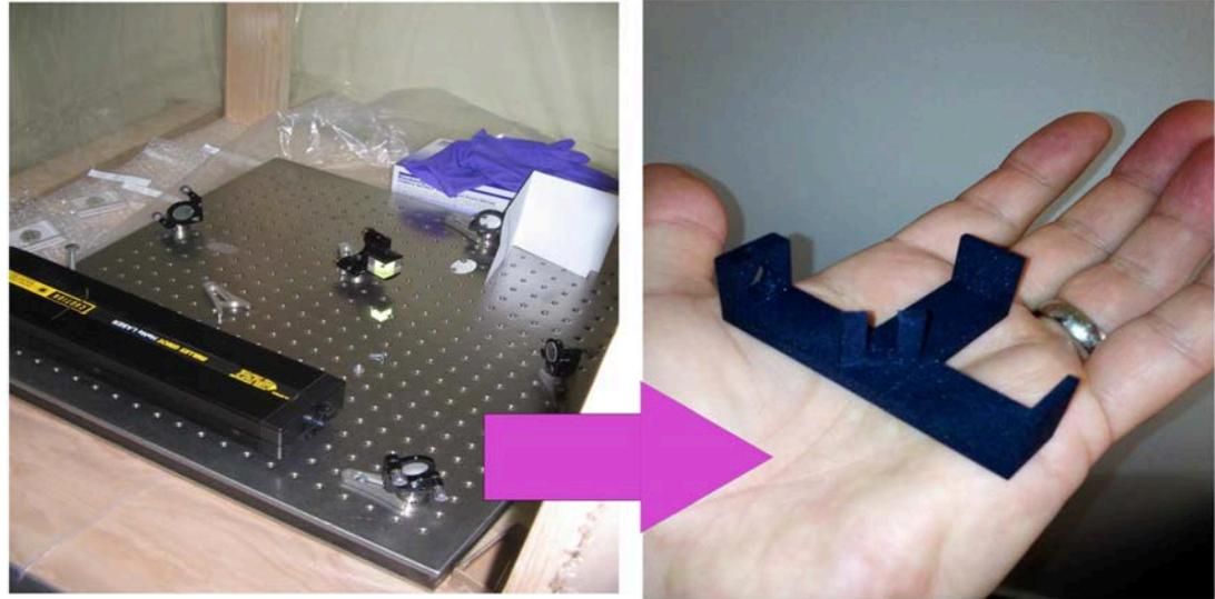
HeNe Interferometer built on a 23" optical board (left). Equivalent interferometer built using AM. Courtesy of Simon Woodruff, Woodruff Scientific.
