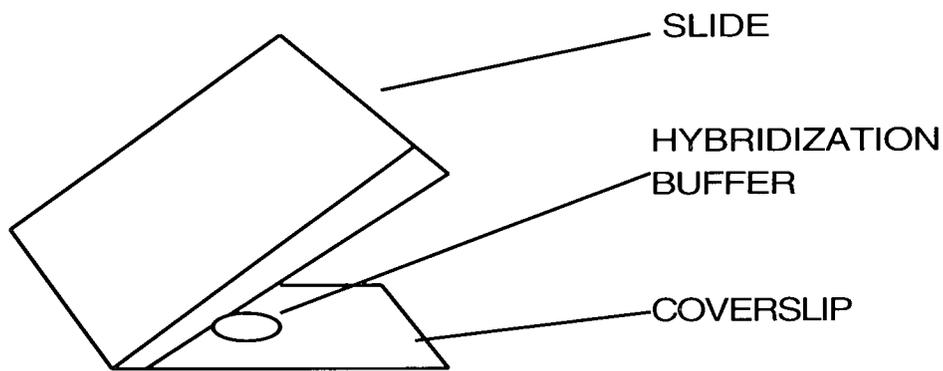
The buffer is applied to the coverslip and the slide is gently lowered at an angle across the coverslip, allowing capillary action to pull the coverslip up to the slide.
