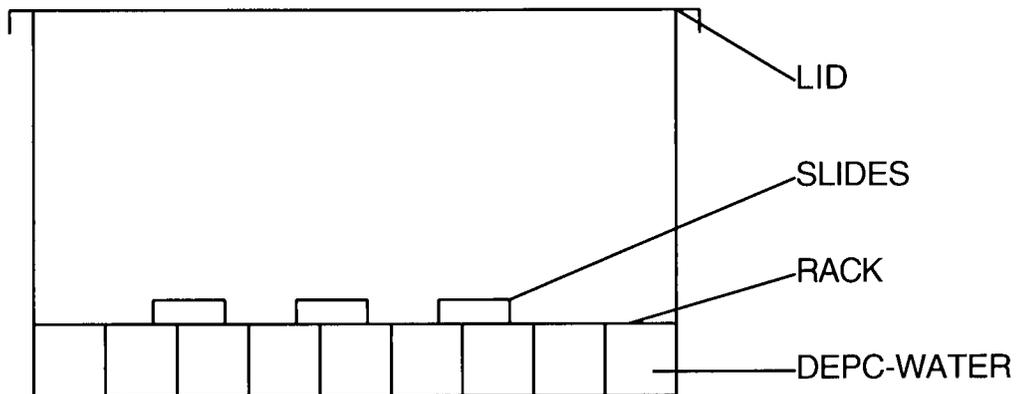
Slides are incubated in a humidity chamber to prevent the tissues from drying.
