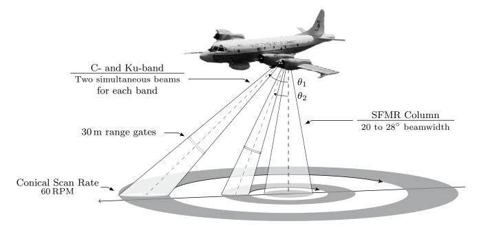
The Imaging Wind and Rain Airborne Profiler (IWRAP). The measurement geometry of the downward-pointing, conically-scanning IWRAP Doppler radar and nadir-viewing SFMR instruments on the NOAA WP-3D aircraft. Angles  $\theta_1$  and  $\theta_2$  denote the outer (~40°) and inner (~30°) beam tilt angles, respectively. The IWRAP radar is well suited for studying the boundary layer and complements additional remote sensing and in situ measurements aboard the P3 aircraft for studying hurricanes.
