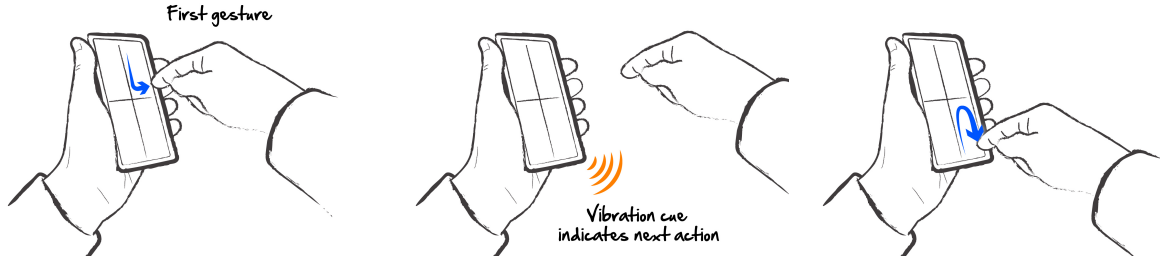
Figure 2: Example of first three steps when entering H4Plock. The user is presented with a vibration cue after entering a gesture, to indicate whether the following gesture to be entered should be selected from the primary or secondary passcode. This process will continue until up to a total of four gestures have been entered.
