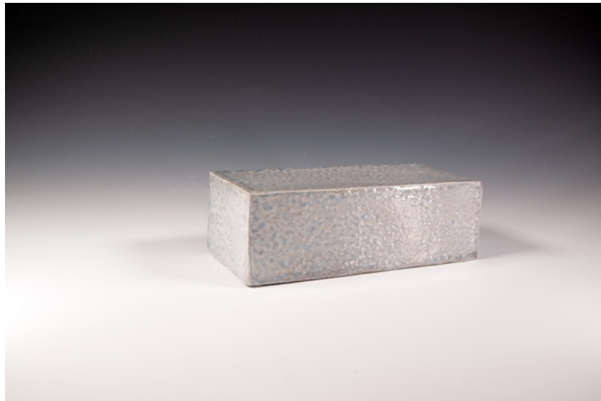
Figure 5: printed RGB glaze pattern completely obscured by soda.
