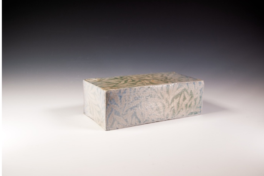
Figure 6: printed RGB glaze separating into blue and green.
