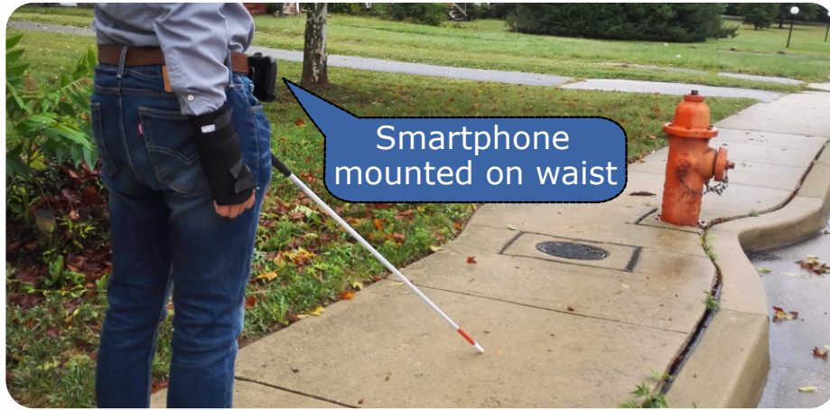
FIG. 6.6: Prototype of the front-end system, RTVision. It is implemented in a generic smartphone and utilizes the camera, the GPS sensor which is used to trigger the camera, and the Wi-Fi module used to download the contextual database (Li et al. 2017).
