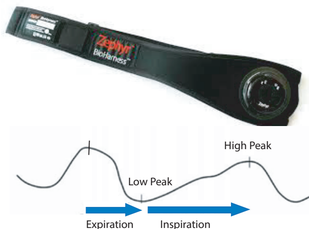
FIG. 4.1: Zephyr bio-harness sensor can sense the change in the tidal volume of a human chest during inspiration and expiration, which can help to identify breathing patterns.
