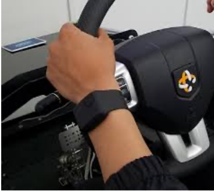
Figure 19: Driver wearing E4 Wristband for vital health data attributes
