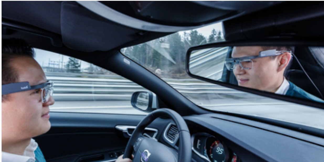
Figure 18: Driver wearing Tobii Eye Glass 2 for Distraction data attributes
