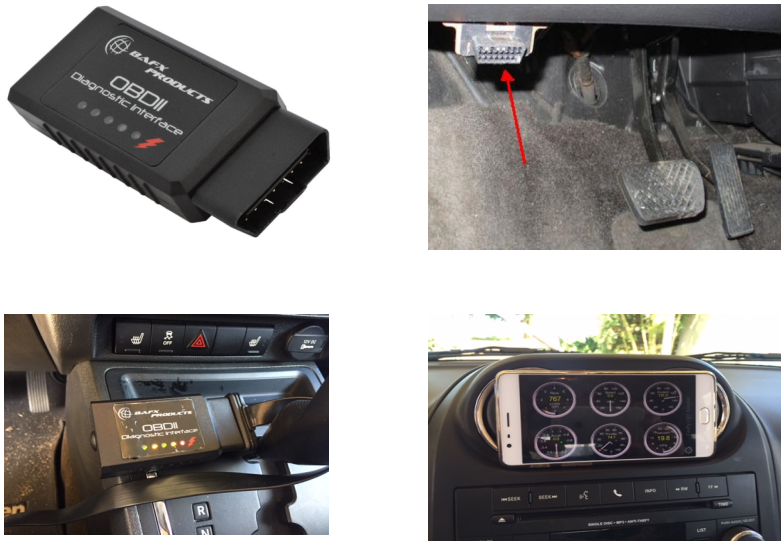
Figure 11: Telematics data Collection Mechanism
