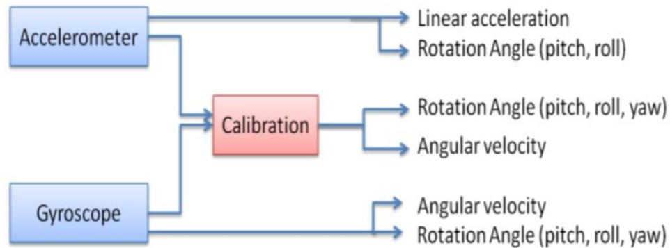
FIG. 2.1: An IMU sensor with accelerometer and gyroscope
