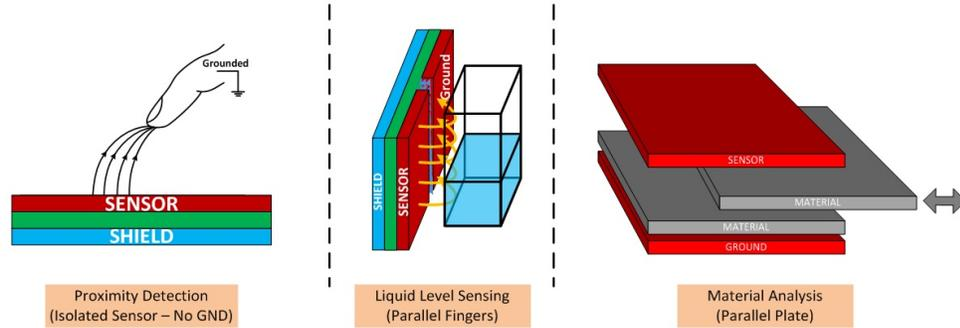
FIG. 2.2: Various Topologies of a capacitive sensor with its applications
