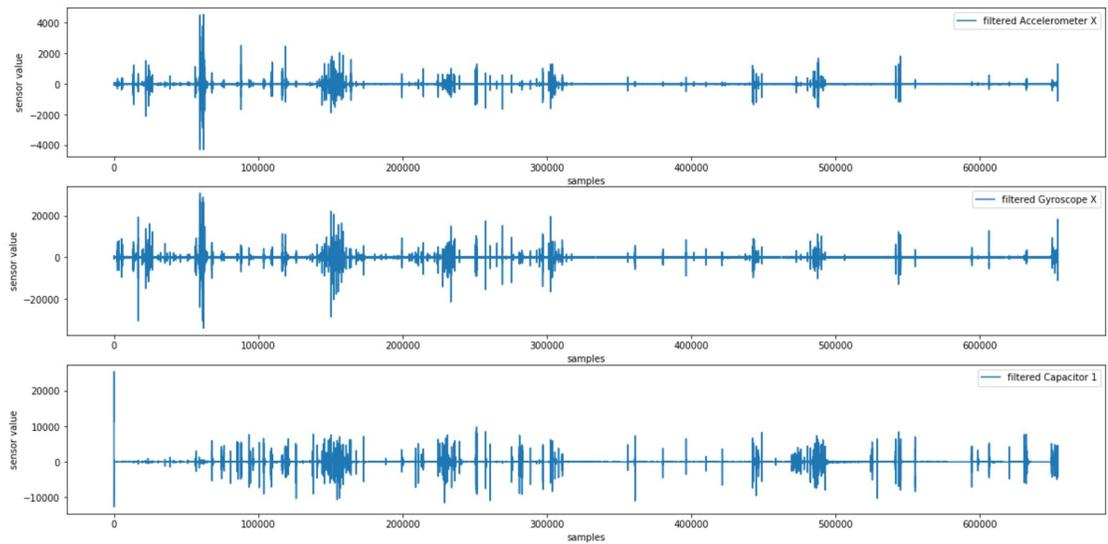
FIG. 4.10: BandPass Accelerometer-X, Gyroscope-X, and Capacitive-1 sensor values of RZ0017
