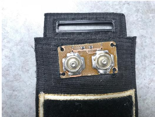
FIG. 3.4: Sleep lab RestEaze band with Sync Signal
