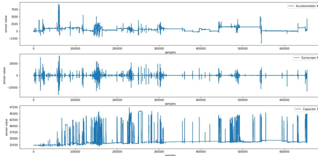
FIG. 4.9: Raw Accelerometer-X, Gyroscope-X, and Capacitive-1 sensor values of RZ0017
