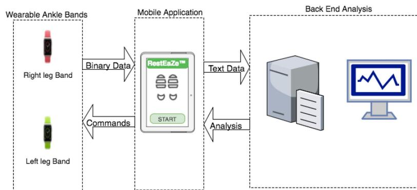
FIG. 3.1: Architecture of RestEaze System
