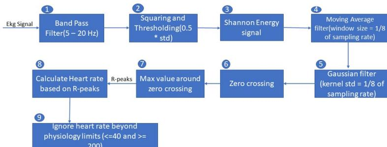
FIG. 4.4: Block Diagram for finding Heart Rate
