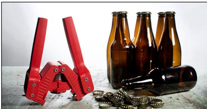
The red device to the left is a homebrewers hand-capping tool. It clamps onto a metal cap and curls it to make a tight seal onto a bottle.
