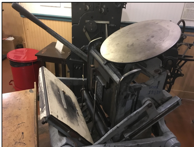
Old-fashioned printing press c. 1905, courtesy of the Baltimore Museum of Industry. A piece of paper goes on the large rectangle piece and ink goes on the large circle pad. A roller rolls ink onto the pin and inks the design onto a piece of paper on the rectangle piece.
