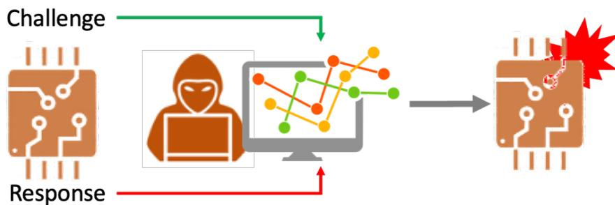
Figure 4.1: Threat model for CRP-based modeling attacks in which an attacker collects CRPs, creates a model, and then deploys said model to exploit the IC.
