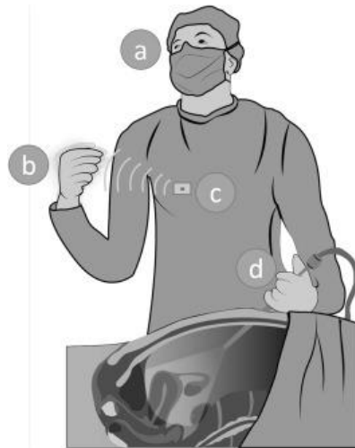
Fig. 1. 6. One hand interaction: viewing the image (a), performing a gesture (b), RadSense worn on chest (c) busy hand holding tool (d).
