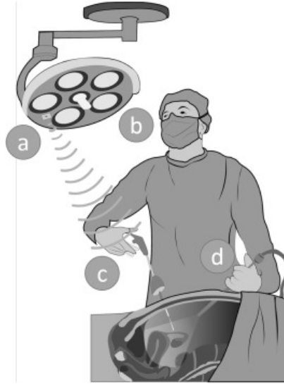
Fig. 1. 7. No hands interaction: RadSense attached to medical light (a), viewing image (b), performing finger gesture while holding a tool (c) busy hand holding tool (d).
