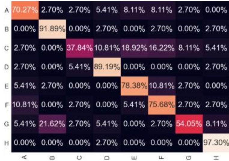
Fig. 1. 39. This figure shows the confusion matrix results using the original data set with a total of 74% accuracy. The labels for the 8 medication tampering methods are as follows: A is Move Bottle Lid, B is Shake Bottle, C is Move Bottle, D is Move Pill Hand, E is Move Pillbox, F is Move Pill in Box, G is Move Pillbox Lid, and H is Move Pill in Blister Pack.
