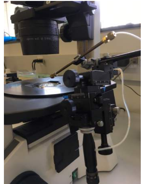
Close-up of injection needle holder with glass slide on compound microscope.
