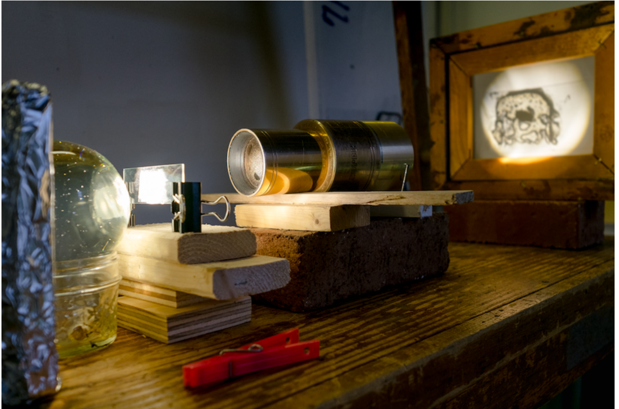
Figure 7: Constructed projector with microscope slide as subject, in studio
