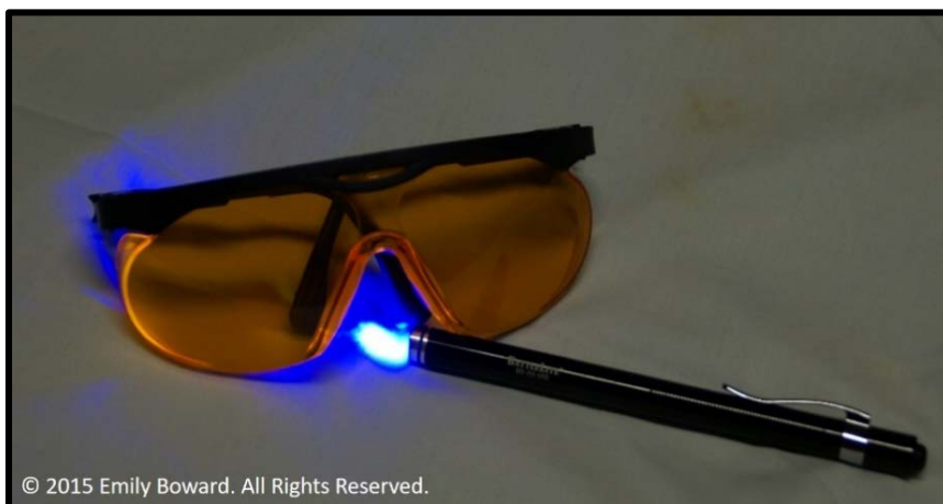
Figure 38. Orange filter glasses and MicroBlue II™ 455nm ALS used for viewing suspected stains (Fish et al. 2014, Lynn Peavy Company 2012).
