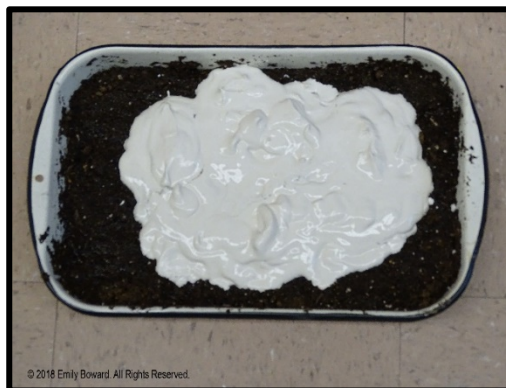
Figure 52. Plaster of Paris mixture poured onto shoe impression.
