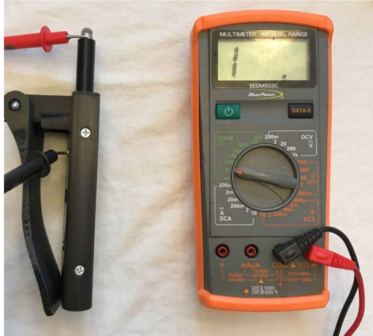
Figure 54: Testing the continuity to ensure proper touchscreen insert operation.
