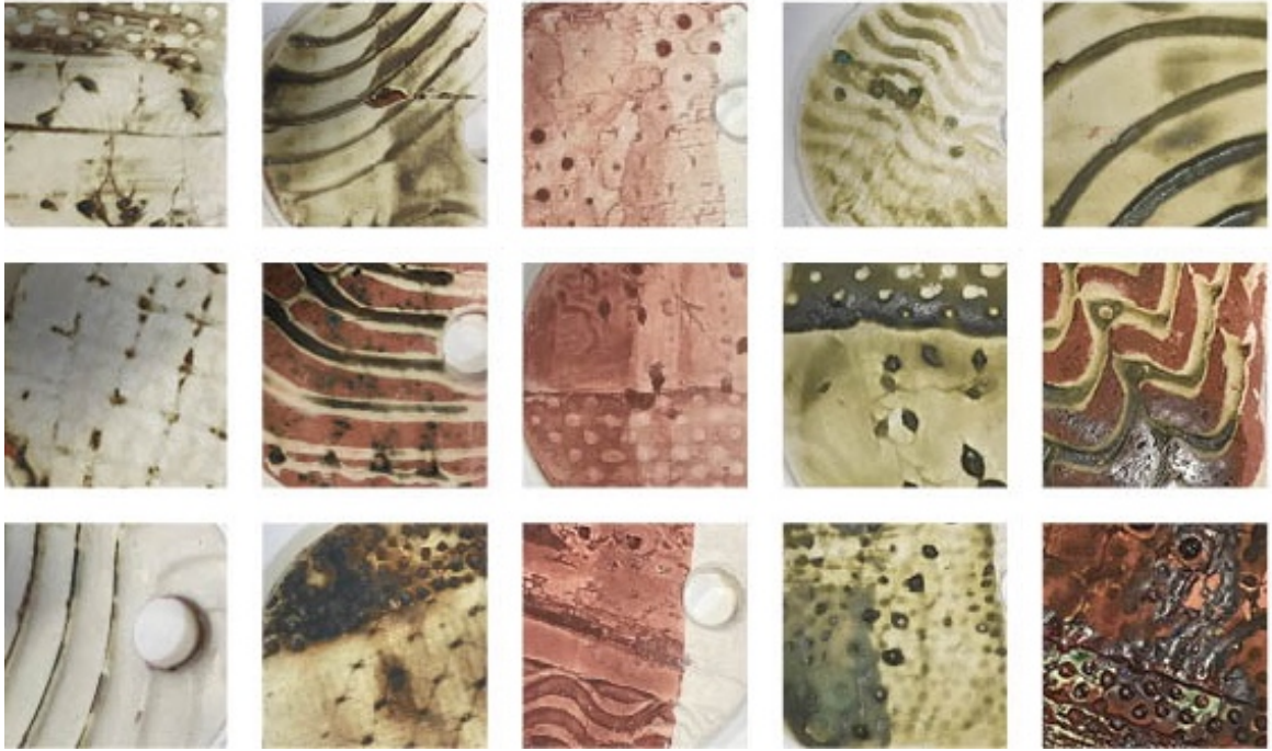
Figure 55. These close-ups show the results of the various oxide washes by vertical row: Black Copper Oxide, Red Copper Oxide/ Gertsley Borate, Red Iron Oxide/Gertsley Borate and Copper Carbonate/Gertsley Borate twice.
