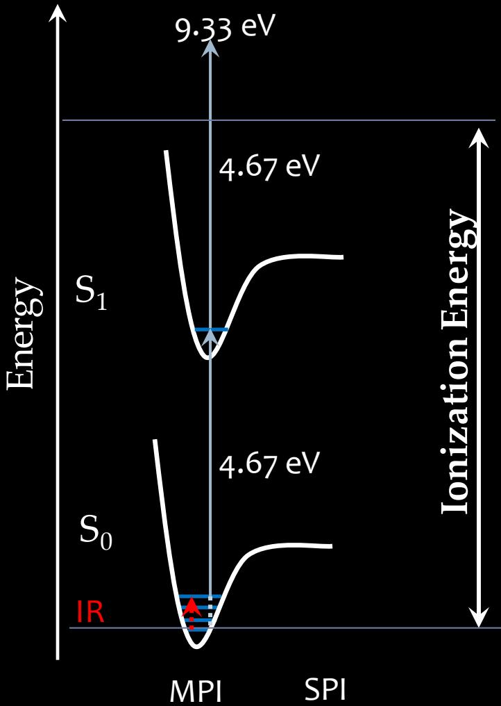
Resonance Enhanced Multiphoton Ionization
